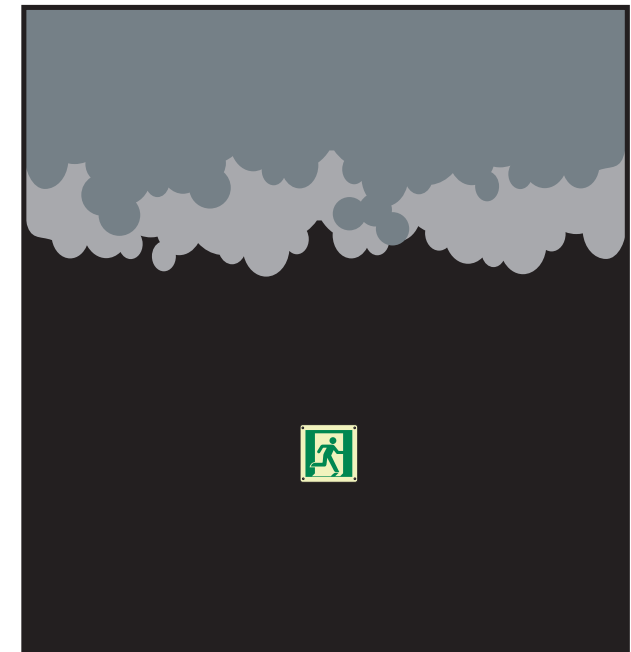
Standard sign and floor proximity exit sign Smoke and failure of lighting
